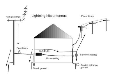
Another path for lightning, common with taller towers or underground utilities, is from the tower through equipment to power mains, telephone, and/or CATV lines. Water and gas lines can be included in the path.
