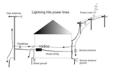
One path for lightning, common with above ground utilities and modest antenna heights, is from power lines to the house and tower grounds. It can also loop from mains through telephone and cable equipment, or the cable and telephone can also share bringing lightning energy into the house.
